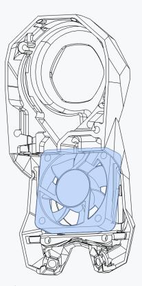
Insert the fan at a slight angle and clip it into place.
