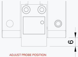
The position can be fine-tuned later. Set an initial position of about 6mm below the plastic part.
