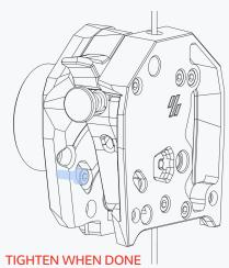
Don't forget to tighten the second motor bolt after adjusting.
