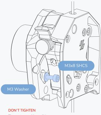
The motor position will be adjusted in the next steps. Don't fully tighten just yet.
