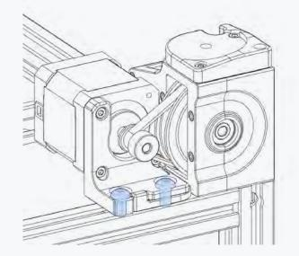
**TIGHTEN BOLTS** After closing the tensioner the M5 bolts can be properly fastened.
