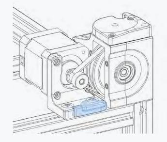
**CLOSE THE BELT TENSIONER** Flip the belt tensioner latch closed.
