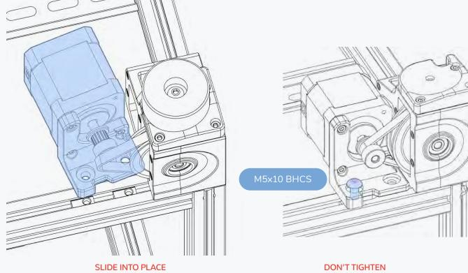
Insert at an angle and slide into place.
