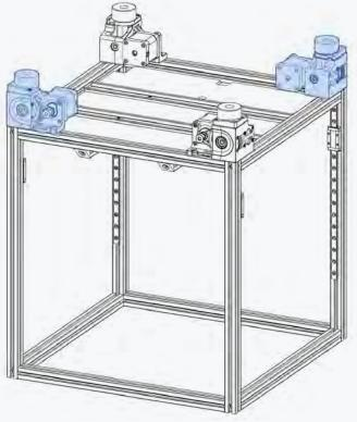
**REPEAT INSTRUCTIONS FOR THE MIRRORED DRIVES** Build two more Z drive following the instructions that came before. The printed parts are mirrored.
