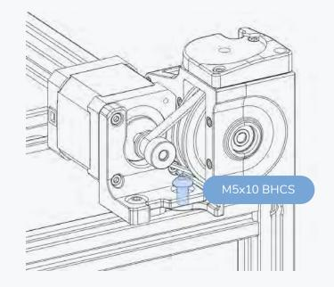
DON'T TIGHTEN Leave the bolt loose for the next step.
