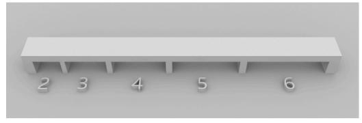
Minimum Hole Diameter and Engraved Detail Width, Z-Axis, at 0.05mm Layer Height
