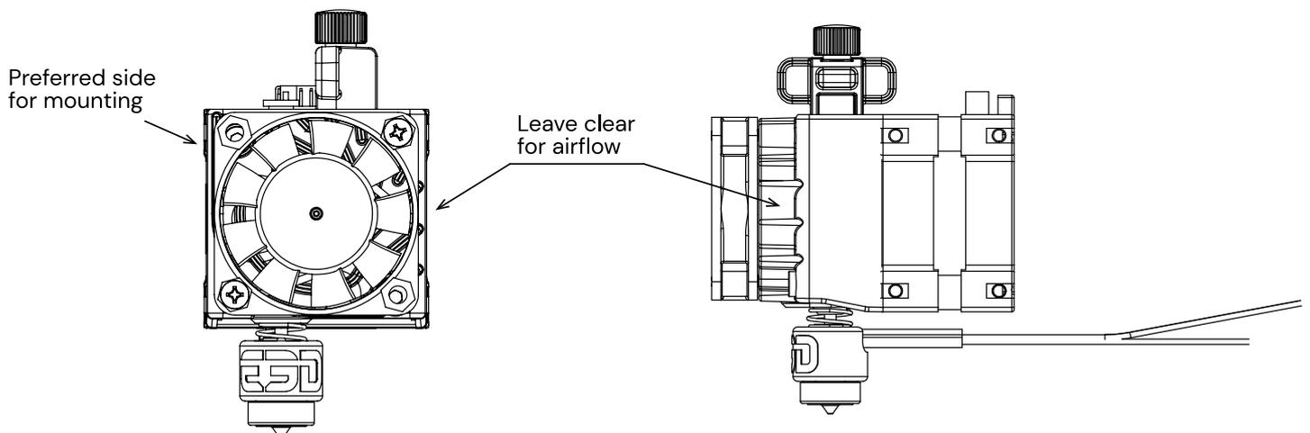
Hemera is mounted to a flat surface via the T-slots on the left or right sides of the motor. Typically Hemera is mounted onto the left side, as the air from the heatsink cooling fan exits on the right. If mounting on the right, ensure that sufficient space is left for airflow.
