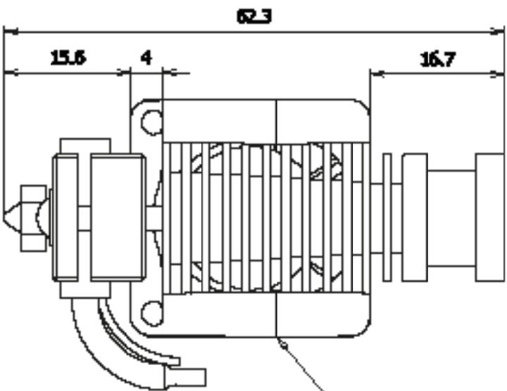
NOTE: THE DUCT CAN BE MOUNTED EITHER WAY UP
