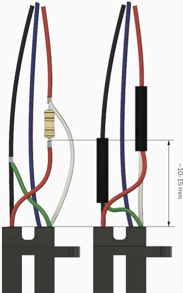
**HOW TO CONNECT THE WIRED OPTICAL SENSOR**
