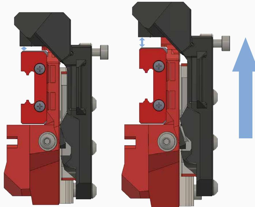
Magnetic and gravitational forces keep the toolhead from shifting during printing. If the nozzle contacts something solid (like the bed), the black section of Tap and toolhead move up, and the optical sensor will trigger. There are stops built in to prevent it from moving too far, unless you really want the front to fall off.
