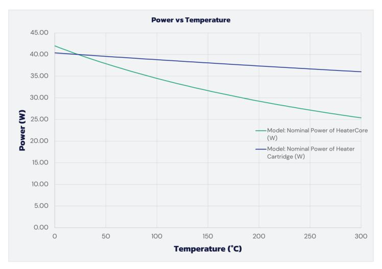
Initial Resistance of a 24V heater at  $23^{\circ}$ C:  $14.4\Omega$  Temp Coefficient of Heater Core: 0.002078 Temp Coefficient of Heater Cartridge: 0.002078
