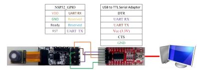
The following table shows the general pin connections between NSP32 module and the adapter.
